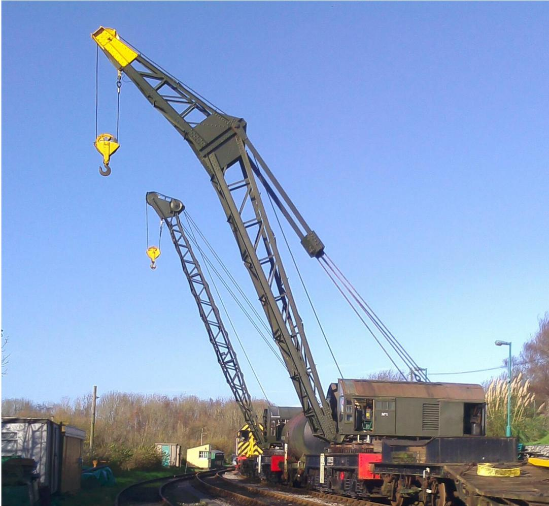
The two cranes which are often seen in the siding opposite the platform at Norden Station were built in the late 1940s and early 1950s by Stothert and Pitt of Bath for use at the Southampton Docks. These cranes are known on the Swanage Railway as FBC1 and FBC2 but officially the makers numbers are CB5968 No1, 15 ton; and CC1011 No1 10 ton, respectively.
